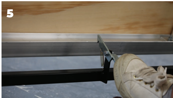
Release the MELBA Catch by Foot before lowering the Units.
