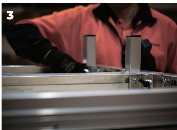
Insert 4 Longest Podium Legs into Corner Brackets and hand tighten Wing Bolts.
