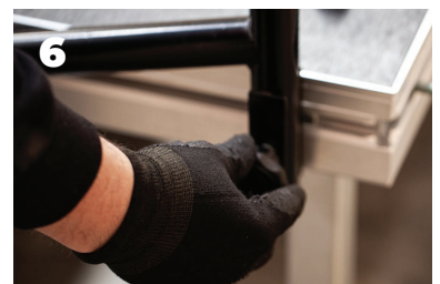
Add Hand Wheels and Hand Tighten once all Hand Rails are correctly in place.
