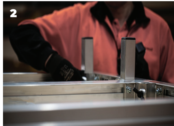
2 Hand Tighten Wing Bolts so Legs are Secure.
