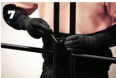
When all Hand Rails are secured, add Hand Rail Clamps. Use Rail Clamp Allen Key to securely tighten the Rail Clamp Bolt. All Rails should be joined to each other.
